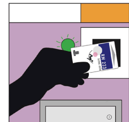
Swiping key card will cover the LDR blocking light from entering. The traffic light system indicates green for go and the machine can be used
